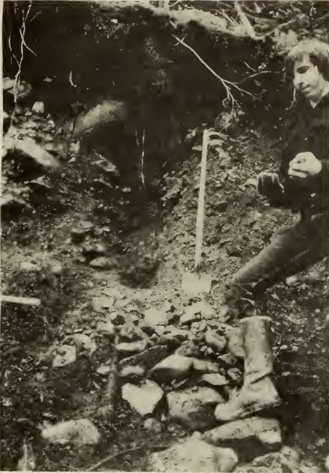
FIGURE 6. Typical channel sample used for evaluating placer deposits.
